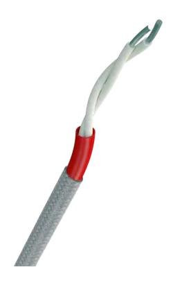
Signaline Linear Heat Detector can detect a build-up of heat anywhere along its length. When any point along the length of the cable reaches a predetermined temperature an alarm is initiated.
