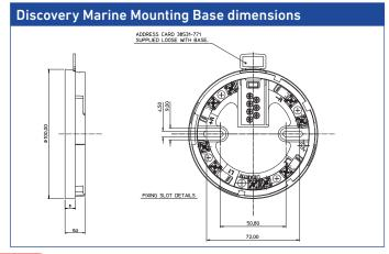
**Note:** Should be used with Deckhead Mounting Box - Part No. 45681-217 if ingress protection is required
